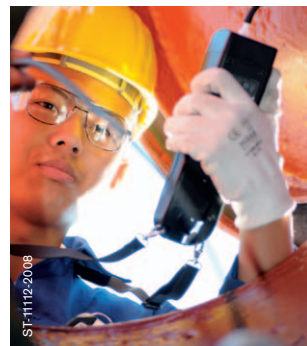
Dräger X-am 5000 Optional external pump for clearance measurements
