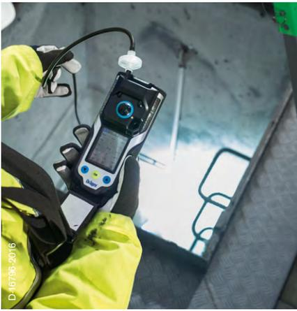
Anyone involved in maintenance or repair work in confined spaces must be accompanied by a competent safety official, valid measurement technology, protective clothing and an emergency plan.
