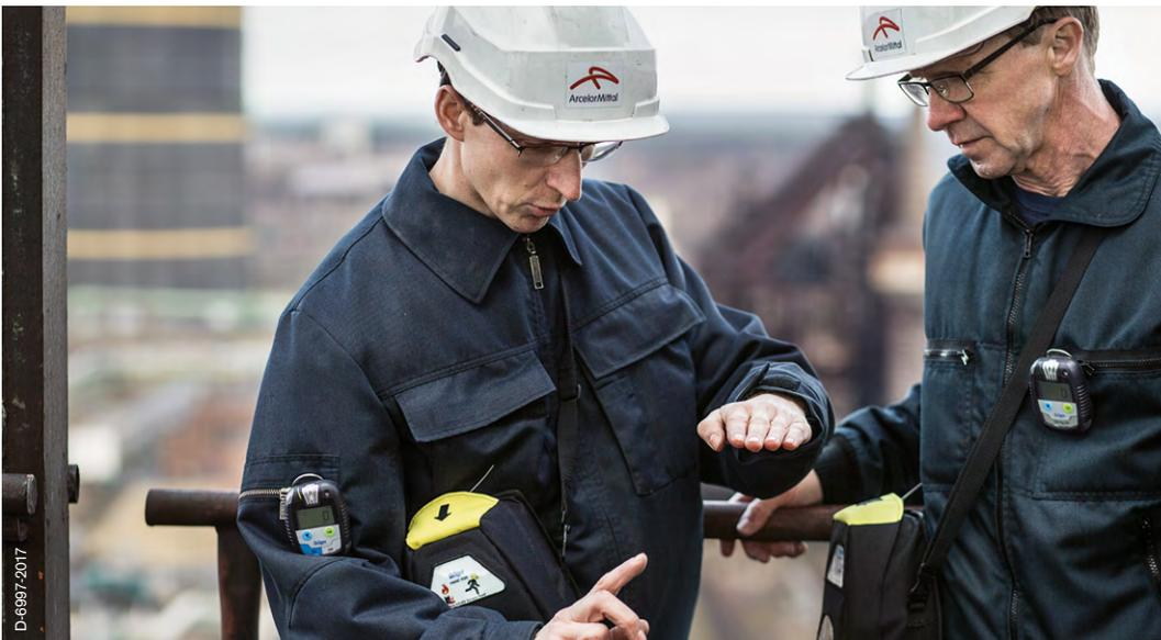
A portable, personal, multi-gas measuring device protects workers in the steel and metal industry from harmful concentrations of hazardous substances.
