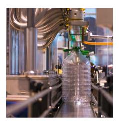
Carbonation of beverages is a proven method for extending the shelf life of drinks. The application of carbon dioxide (CO<sub>2</sub>) under cooling and overpressure gives soft drinks their pleasant fizzing effect.
