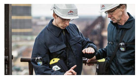
A portable, personal, multi-gas measuring device protects workers in the steel and metal industry from harmful concentrations of hazardous substances.
